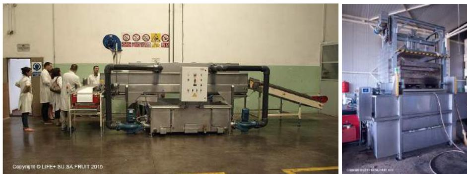
*Fig. 2. Prototypes of thermotherapy machines developed by project partner XEDA*
